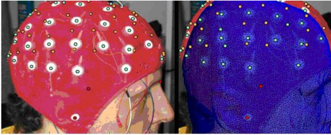
Figure 1. The sensor configuration is derived with the help of a photogrammetric procedure, which consists in marking all the electrodes visible in a set of pictures taken immediately after the EEG acquisition is finished (one picture is shown in the left panel). Triangulation between the two-dimensional projections of each electrode onto the plane of the pictures provide their three-dimensional position. Matching the craniometric repere points, allows to express these positions in the same coordinate system as the head model derived from MRIs. Superimposition of the head model as seen from the camera position with the picture (right panel) offers the oportunity to visually check the accuracy of the alignment between sensor positions and BEM.
