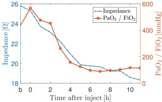
**Figure 5:** Absolute value of the measured impedance at configuration #1 at 70 kHz (blue) compared to the Horowitz-index (red). The time after Lipopolysaccharid-injection is shown on the x-axis. "b" denotes the baseline measurement. 3 hours after injection, an ARDS was diagnosed ( $\text{PaO}_2 / \text{FiO}_2 < 300$ ).
