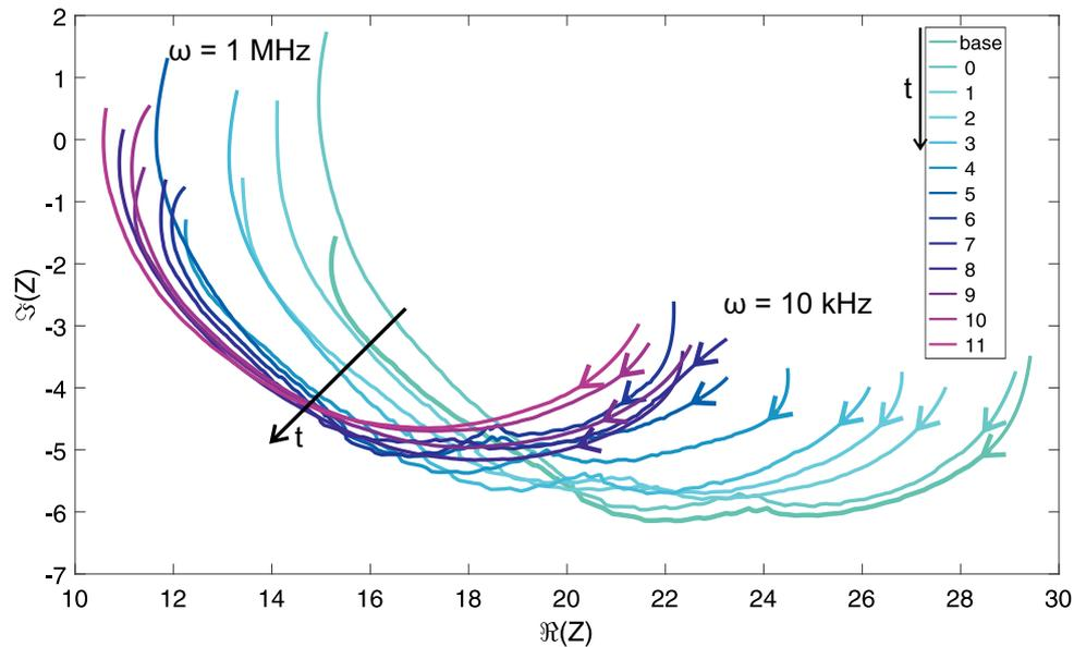
**Figure 7:** Results of the Bioimpedance Spectroscopy (BIS) measurements at configuration #1 (see Tab. 1). Both the real and imaginary part is shown as a function of the frequency. BIS was recorded at an hourly rate. A stable ARDS was diagnosed at  $t=3h$  (see Fig. 4.)
