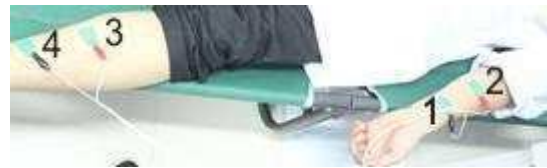
Figure 1 The driving electrodes 1 and 4 inject the stimulus while the voltage dropping across the body was monitored by the electrodes 2 and 3.
