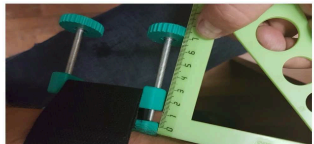
Figure 4: Electrode system pressing control mechanism
