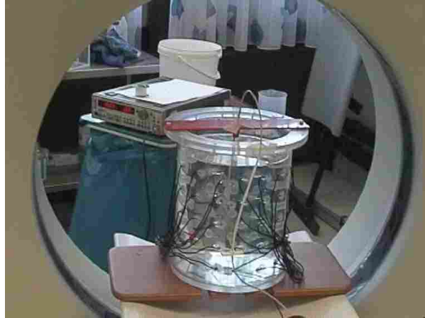
Figure 20. The phantom to localize the electrode positions on the balloon catheter. The phantom stands inside the CT and the catheter is fixed inside the phantom. In the background, there is the function generator to apply the voltage.
