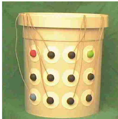
Figure 26. Phantom with 12 electrodes. A four electrode string catheter is inside during the x-ray measurement.
