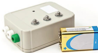
Figure 1. The EEG-to-ECG adapter compared to a standard 9 V battery.
