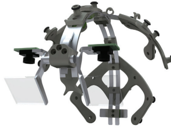
Figure 1. EEG signal acquisition system combined with eye tracking. EEG signals for the SSVEP paradigm are acquired from the visual cortex area and for ERD/ERS from the motor cortex area.
